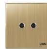
Q9G-2TV 356.000 VND 2 Tivi Socket 1. Impedance: 75 Ω 2. Insertion Loss: VHF < 3.5dB UHF < 5dB, Flatness in band ±1.0 dB 3. Plastics: PC - Box: 10 set - Carton: 100 set Size: 86mm x 86mm
