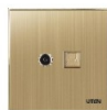
Q9-TVPC 385.000 VND 1Tivi & Computer Socket TV: 1. Impedance: 75 Ω 2. Insertion Loss: VHF3.5dB UHF < 5dB, Flatness in band ±1.0 dB 3. Plastics: PC - Box: 10 set - Carton: 100 set COMPUTER: 1. Temperature: -20 ~ 70°C 2. Insertion Resistance: ≥ 500mΩ 3. Electrical Specification: ELA/TIABI 4. Connection Mode: T568A, T568B 5. Plastics: PC - Box: 10 set - Carton: 100 set Size: 86mm x 86mm
