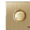
Q9G-1D/S 438.000 VND Speed Control Switch 1. Working Voltage: 220V ~ 50Hz 2. Load Power: 25 ~ 100W 3. Minimum Starting Voltage: 90 ~ 110V 4. Load can be connected: Ceiling fan 5. Never connect the zero line 6. Plastics: PC - Box: 6 set - Carton: 60 set Size: 86mm x 86mm
