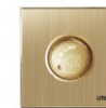
Q9G-1D/Y 486.000 VND Door bell switch Size M 1. Signal frequency range: 100Hz ~ 20KHz 2. No Less than 500 MΩ 3. Maximum load power: 80W 4. Plastics: PC - Box: 8 set - Carton: 80 set Size: 86mm x 86mm
