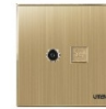
Q9-TVTEL 338.000 VND Tivi & Telephone Socket TV: 1. Impedance: 75 Ω 2. Insertion Loss: VHF < 3.5dB UHF < 5dB, Flatness in band ±1.0 dB 3. Plastics: PC - Box: 10 set - Carton: 100 set Telephone: 1. Temperature: -20 ~ 70°C 2. Insertion Resistance: ≥ 500mΩ 3. Electrical Specification: ELA/TIABI 4. Connection Mode: T568A, T568B 5. Plastics: PC - Box: 10 set - Carton: 100 set Size: 86mm x 86mm
